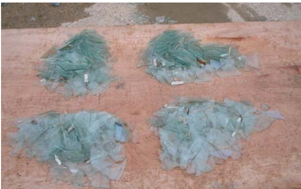
Figure 23. Coning Sample conducted at Viridor Peterborough.
