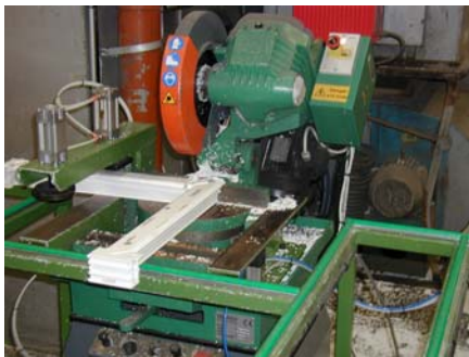
Figure 18. Specialist bench saw used for processing PVC-U frame window waste
