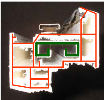
Figure 20. Measuring material volume without including the void space
