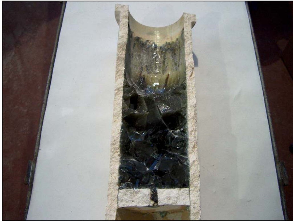
Figure 5. Cross section of the refractory tube used in the smelting trials
