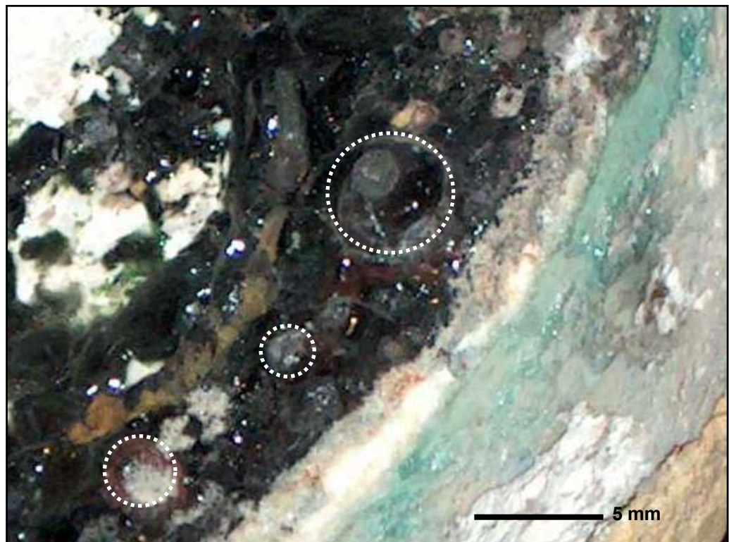
Figure 9. Initial melt, sample GA.6 showing metallic particles at the bottom of the melt
